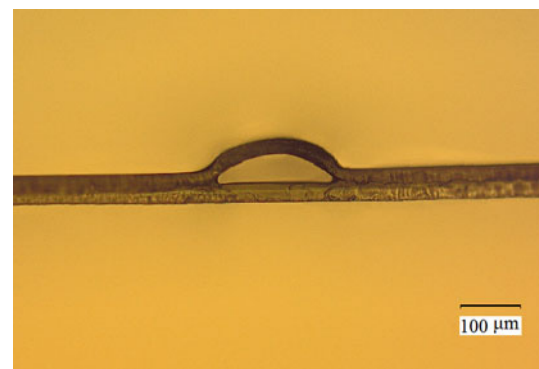
Fig. 14 Cross section of a PS microchannel (channel width 280 \mu\text{m} , channel depth 90 \mu\text{m} , scale bar 100 \mu\text{m} )
