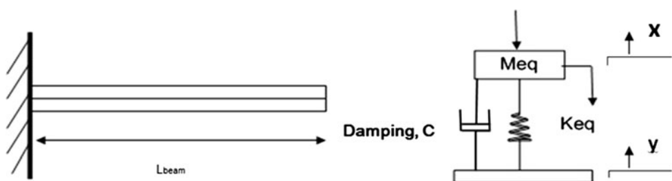
Fig. 3 a Schematic representation of the cantilever beam at one fix end b first order model of a resonant system
