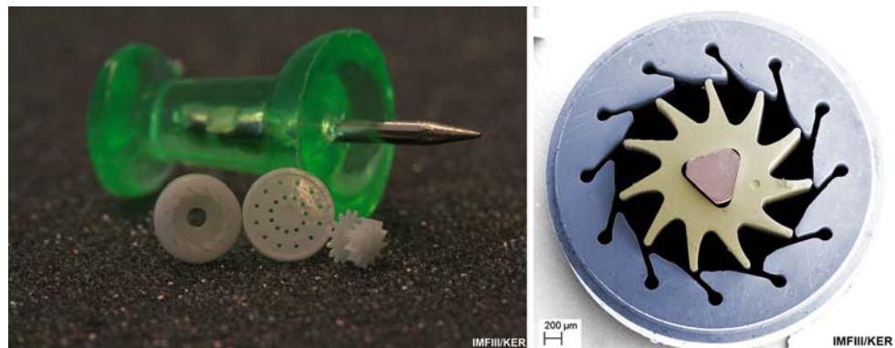
Fig. 12 Comparison of the sintered zirconia parts with a needle pin ( left ) and SEM micrograph of an assembled turbine without the perforated plate ( right )
