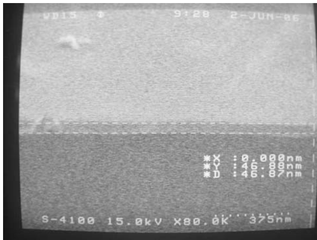
Fig. 12 The thinnest beam to date was 47 nm thick. The sample tilt was 79°
