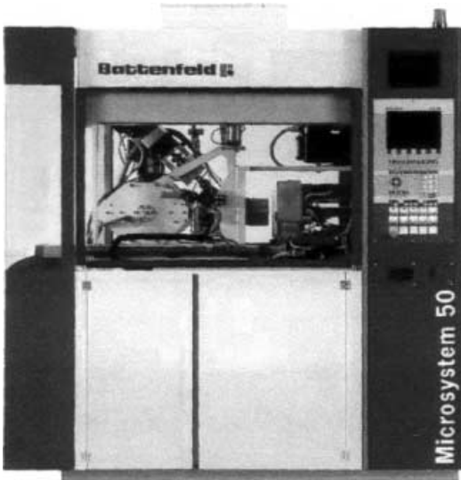
Figs. 1, 2. 50 t injection molding machine with special equipment for micro molding (Ferromatik K 50, top); 5 t micro injection molding machine for minimal shot weights (Battenfeld Microsystem 50, bottom)
