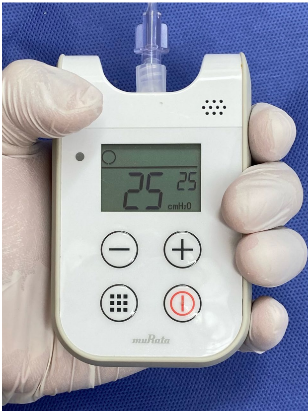
Fig. 1 The SmartCuff (Smiths Medical Japan, Tokyo), an automatic cuff pressure controller
