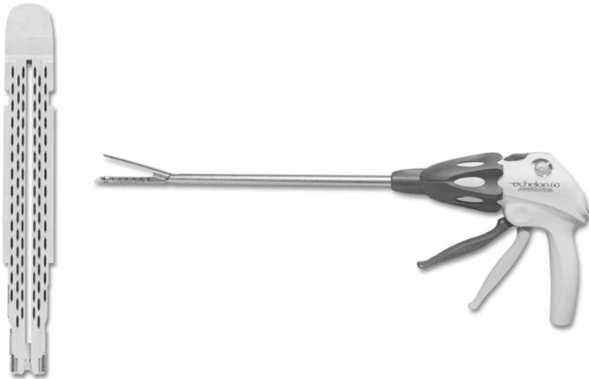
Fig. 1. The endopath stapler (Echelon 60) delivers a true 60-mm staple line and works with a wide range of cartridges including white, blue, green, and gold cartridges. The cartridges have an internal cutting knife, and they can place two triple-staggered rows of titanium staples
