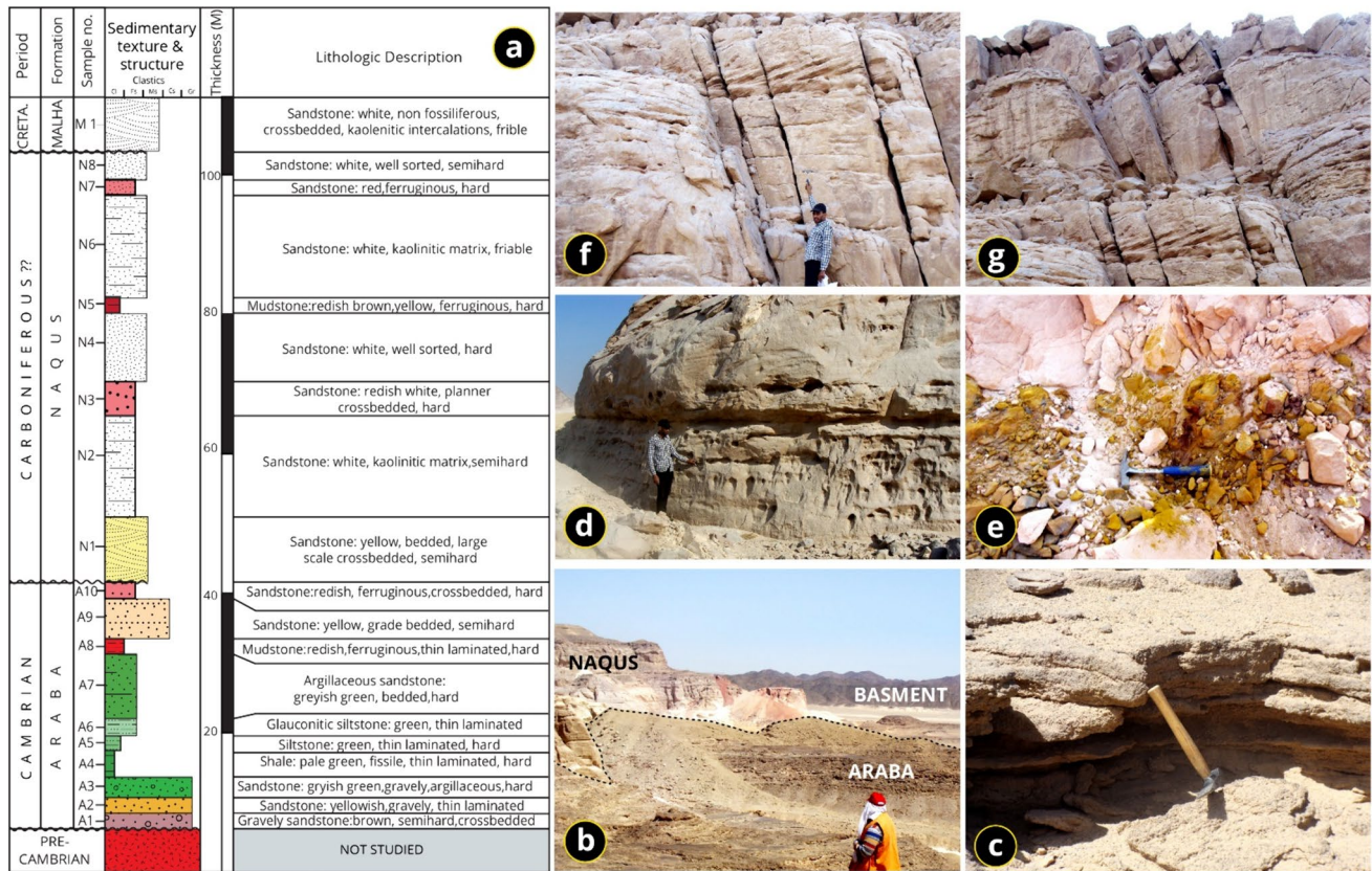
Fig. 2 a A columnar stratigraphic section of the investigated successions in Wadi Dakhl. The figure includes field photographs showcasing the distinctive field characteristics of the Araba and Naqus formations, as follows: b the photograph captures high relief basement rocks and highlights the boundary separating the Araba and Naqus formations. c The image illustrates conglomerates and pebbles found in the lower section of the Araba Formation. d The image displays
