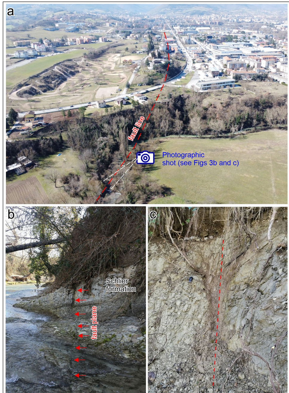
Fig. 3 a Aerial photo (taken by drone) showing the alluvial plain of the Giano river and the fault alignment described in the text: in the background the town of Fabriano. b and c detail of a fault plane affecting the marly-calcareous bedrock (Schlier formation)
