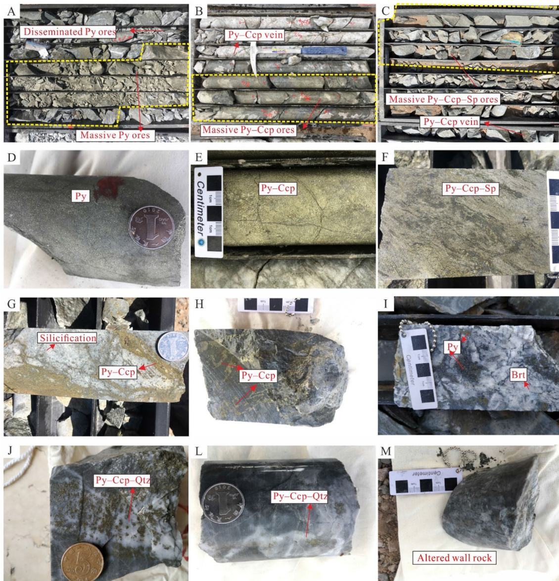
Fig. 5 Photographs of representative ore samples from the Huangtan Au–Cu–Zn deposit. A Massive pyrite ores and disseminated pyrite ore; B Massive pyrite–chalcopyrite ores and pyrite–chalcopyrite vein; C Massive pyrite–chalcopyrite–sphalerite ores and pyrite–chalcopyrite vein; D Massive pyrite ores; E Massive pyrite–chalcopyrite ores;
