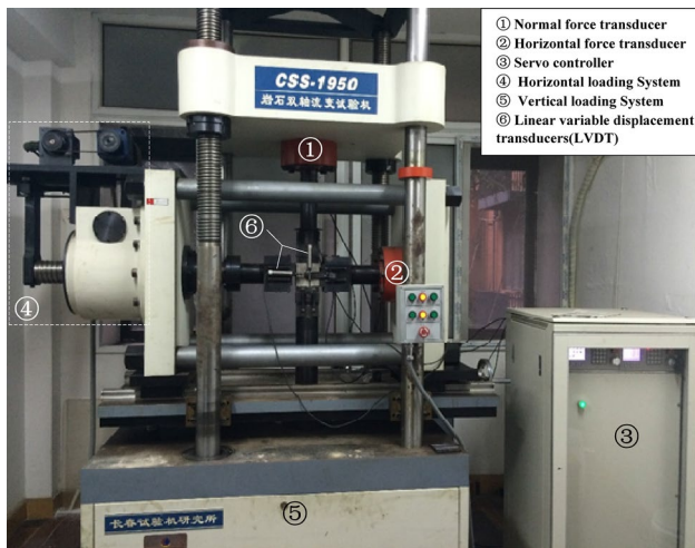
Fig. 1 CSS-1950 servo-controlled rheological testing machine
