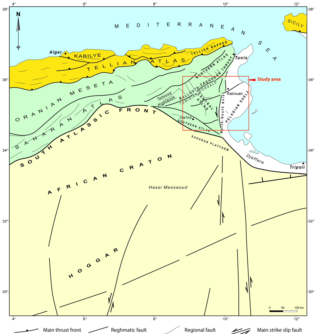
Fig. 1 Simplified structural sketch of the eastern Maghrebian area showing the deformed Atlasic domain to the north of the South Atlasic front, the African Craton to the south with the Hoggar fault system and the location of the study area. Tunisian features are especially delineated
