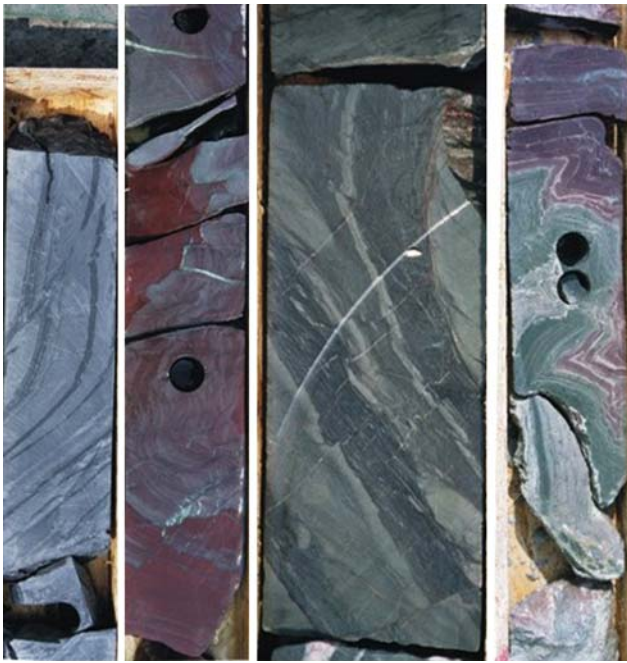
Fig. 14 Cut drill cores from Carboniferous sections in wells from Brońsko gas field confirm the structural style recognised in BR-9 well from dipmeter record (Fig. 12) in showing numerous hinges of metric-scale recumbent folds in sandstone–siltstone lithology, with local, shallow dipping axial-planes and fan cleavage, particularly well developed in the overturned limbs of the folds
