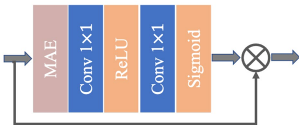
Fig. 4 The structure of MAE-CAU
