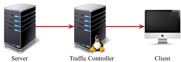
Fig. 3 Experiment testbed. The client consumes video provided by the server, while the traffic controller sets the level of network congestion
