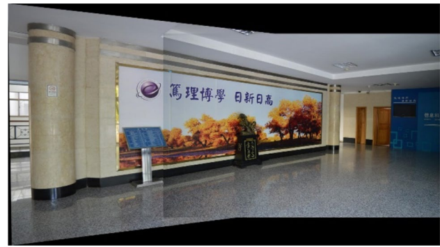
Fig. 8 Stitched image without seam removal
