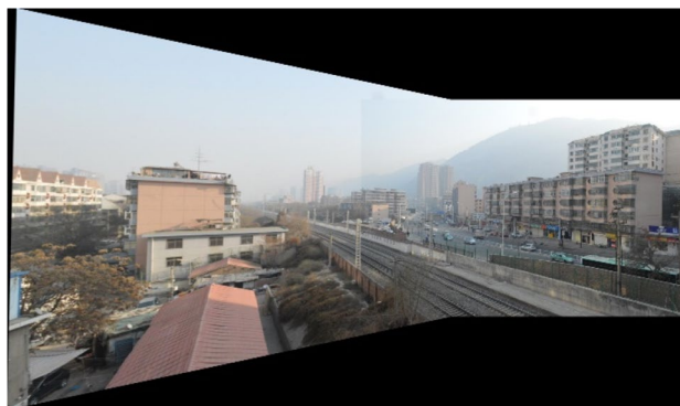
Fig. 11 Stitched image without seam removal
