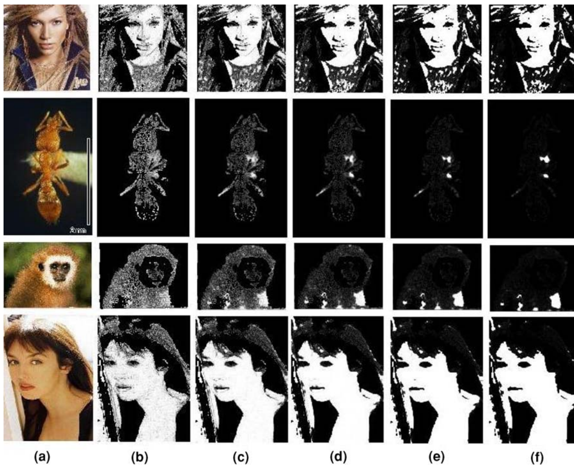
Fig. 16 Convergence of CLA for skin probability map. a Original image. b Combined probability map. Probability map after: c 25 CLA iterations, d 50 CLA iterations, e 75 CLA iterations, f 100 CLA iterations
