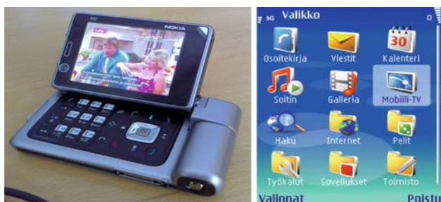
Fig. 3 Left Nokia N92 displaying DVB-H broadcast. Right Mobile-TV application can be found in the phone menu
