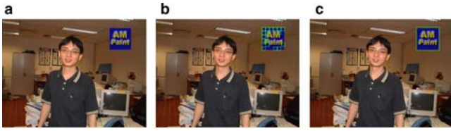
Fig. 4 Region-based detection approach. a Sample frame with logo. b Sample frame with logo-lets detected. c Sample frame with logo detected
