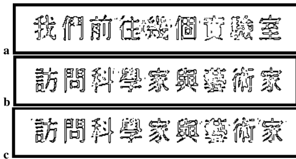
Fig. 6a–c. A pixel that is both a contour pixel and a point in an edge-pair constitutes a foreground pixel in the images
