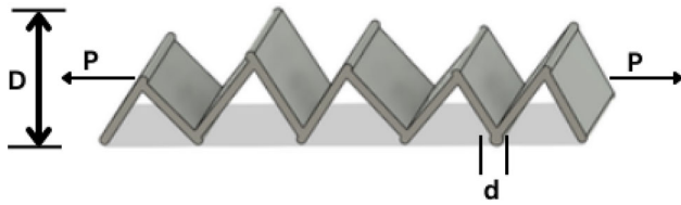
Fig. 14 Tension/compression spring design problem
