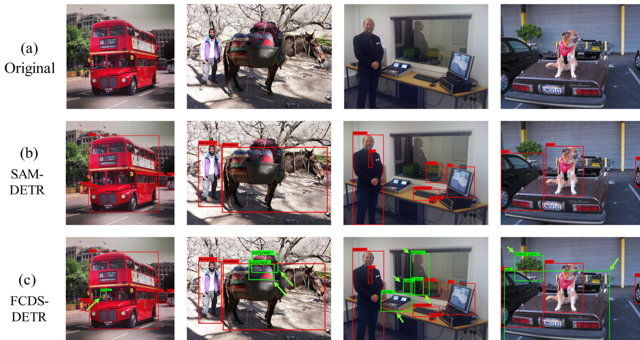
Fig. 8 Detection results of FCDS-DETR and baseline model on COCO dataset. FCDS-DETR can detect small- and medium-sized objects in the image, and the positioning of the bounding box is more accurate
