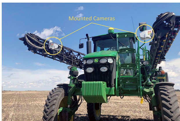
Fig. 2 SWATCAM cameras mounted on each sprayer boom of the field machinery ( https://swatmaps.com )
