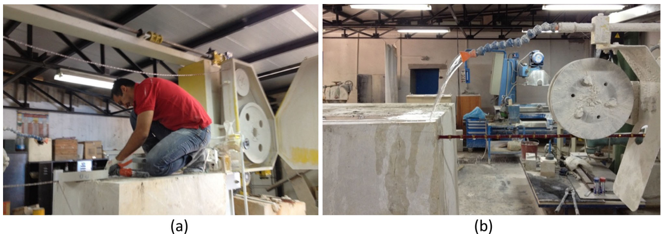
Fig. 2 Mono-wire cutting machine and diamond wire setting (a) and diamond wire in a rock sample, guide pulley of the cutting machine and water feed (b)
