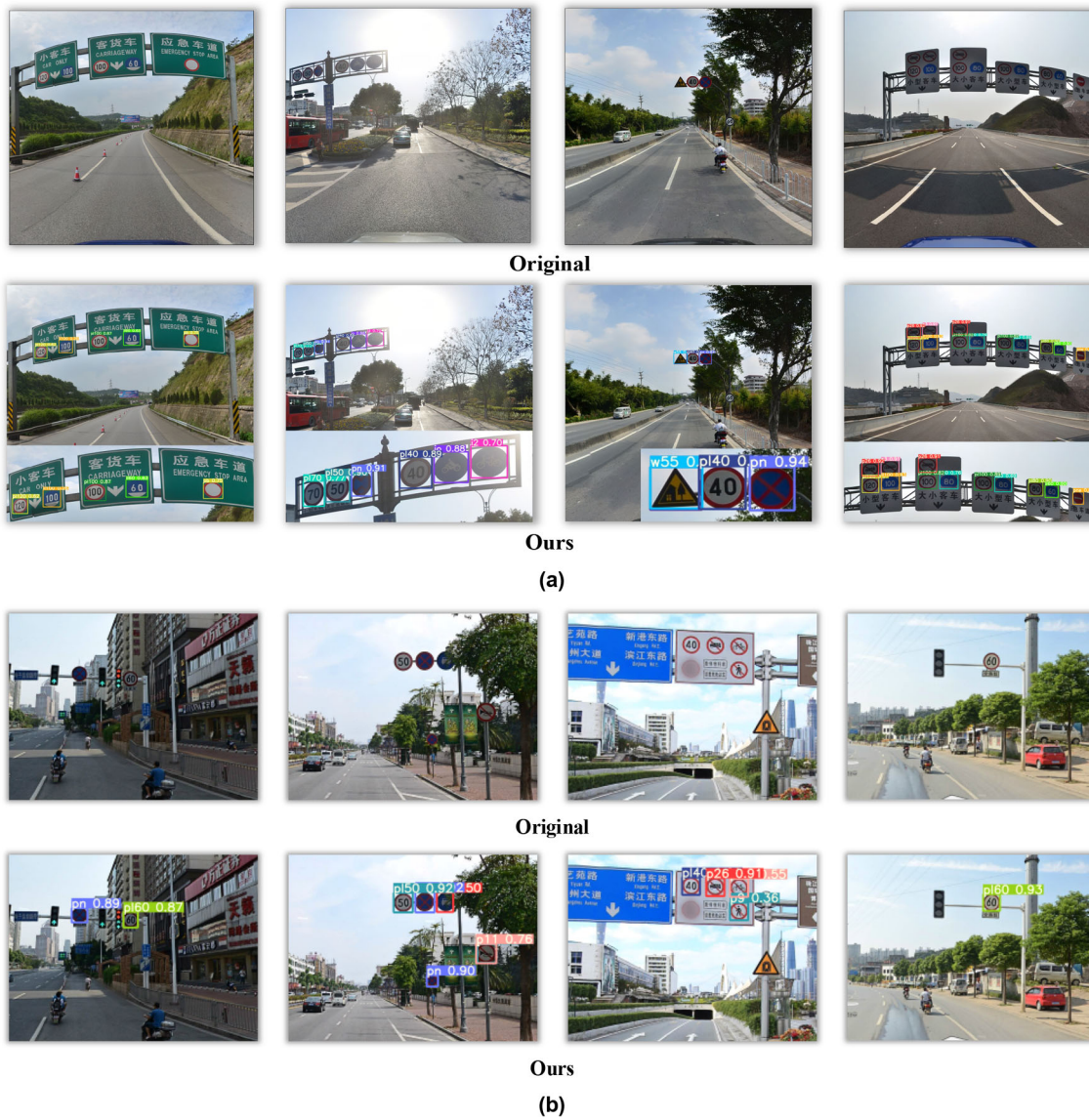
Fig. 10 a Some examples were detected by our method on the TT100K dataset. b Some examples were detected by our method on the CCTSDB dataset
