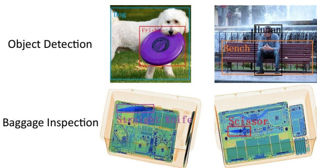
Fig. 1 Illustration of the occlusion difference between prohibited item detection from X-ray images and general object detection. Occluded pixels are unobserved in general object detection, while prohibited items from X-ray images should overlap with other items
