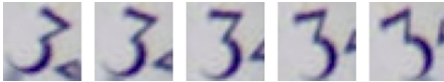
Fig. 1 Fast geometric transformations used to rotate an example image from SVHN data set [20]. From the left: -30^\circ rotation, -15^\circ rotation, original image, 15^\circ rotation and 30^\circ rotation. The precalculated transformations involve filling the image edges based on the
