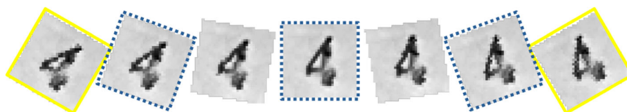
Fig. 6 Sample rotations of a sample image (based on SVHN [20]) from -30^\circ to 30^\circ . Reference representatives of the three neural network branches are marked with dotted lines
