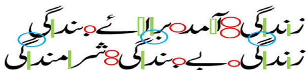
Fig. 8 Red circles and green boxes represent inter-word and inter-ligature variable spacing; sky blue circles show vertical overlapping
