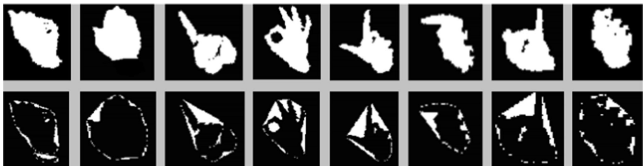
Fig. 12 Convexity defects of the hand shape
