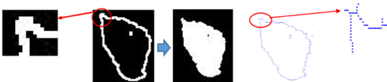
Fig. 5 Thick edge includes several points, image edge detection algorithm, then original image, detected contour, more detailed view are extracted
