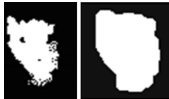
Fig. 2 The binary image before and after morphological operations
