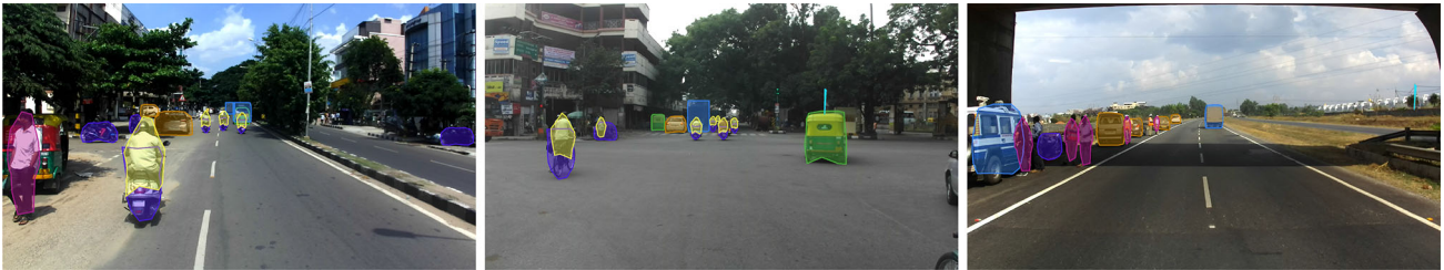
Fig. 3 Examples of Poly-YOLO inference on the India driving testing dataset
