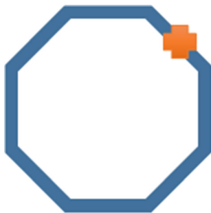
Fig. 4 The eight sensor plates clip together in an octagon formation. Our system uses anomaly detection to determine whether the sensor readings are outside the normal range for the environment. If they are abnormal, then it detects which sensor is giving the most anomalous reading. Here, the north-east sensor is most anomalous and indicates the direction to head
