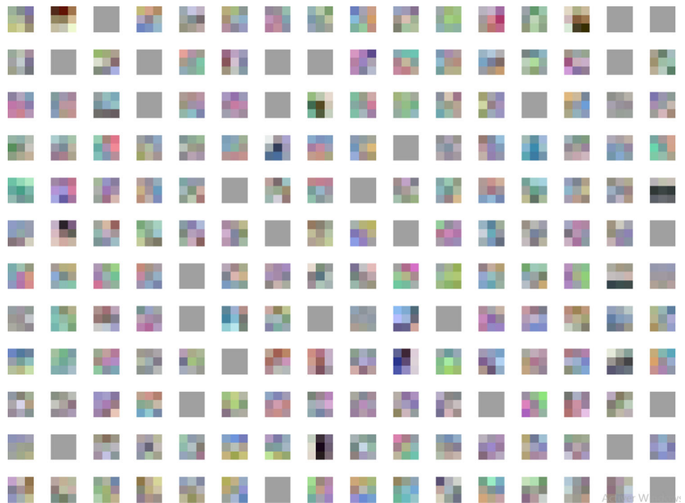
Fig. 12 192 convolution cores of size 3 \times 3 learned by the first convolution layer on the 32 \times 32 input images for the “configuration (D)”
