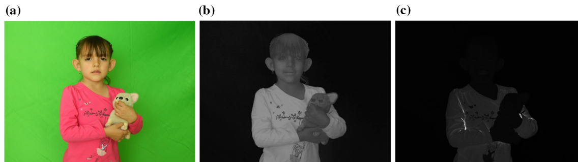
Fig. 4 a Green-screen patch from which two relevant features are extracted; b Euclidean distance between pixel RGB values and the highest intensity green color; c sum of red and blue components over green component (color figure online)
