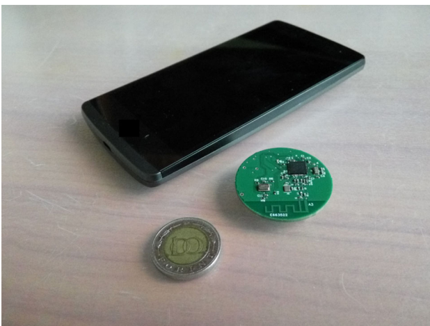
Fig. 2 Size difference between smartphone and a special purpose data collector device (made at University of Debrecen)
