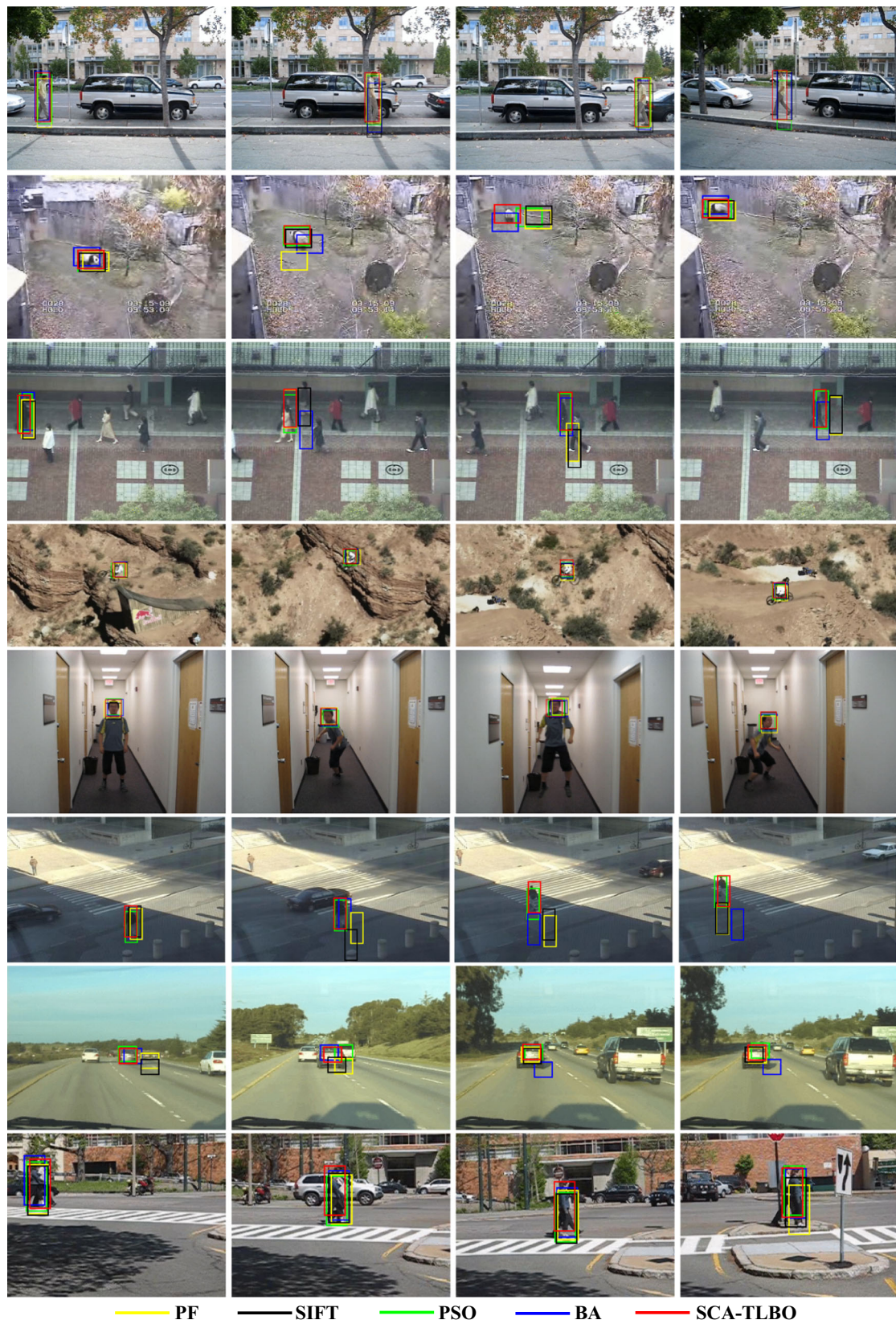
Fig. 11 Tracking result of PF, SIFT, PSO, BA and hybrid SCA-TLBO trackers for David, Panda, Subway, Mountain Bike, Boy, Crossing, Car and Couple Video sequences (from top to bottom)
