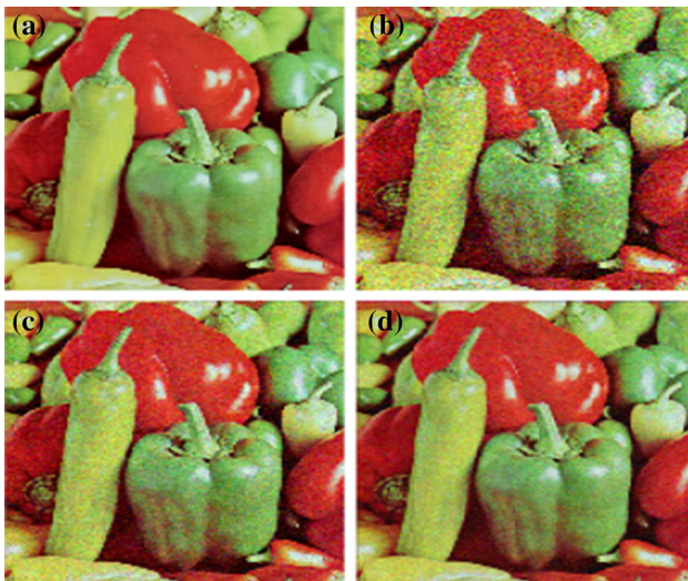
Fig. 5 Experiment with artificial Gaussian noise. Grayscale images “Pepper”. a Original image; b image with Gaussian noise with \sigma = 25 ; c Gaussian smoothing filter; and d FRF proposed filter
