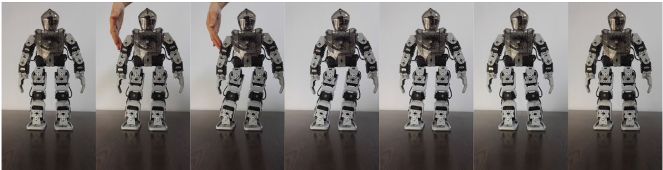
Fig. 17 Snapshots for a biped robot in double-support phase under perturbing external forces
