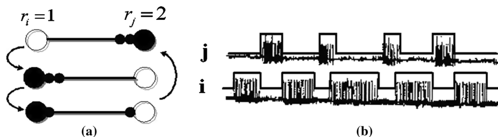
Fig. 3 Mimicking rhythmic patterns generated by CPGs with the SMER dynamics. a Activity of simplified flexor (node n_j ) and extensor (node n_i ) motor neurons during walking of a cockroach and the graph dynamics simulation of its envelope. Here two directed
