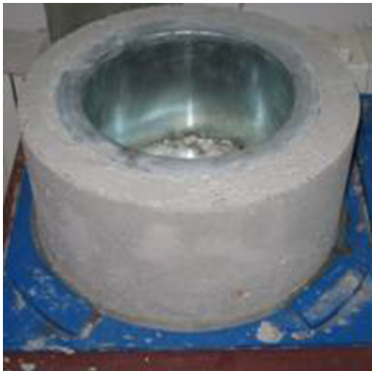
Fig. 3 The ring test setup for restrained shrinkage cracking
