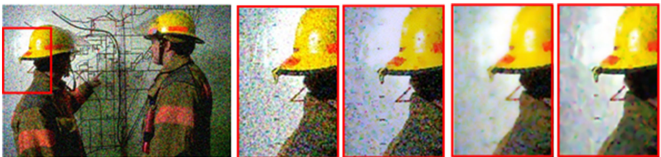
Fig. 20 Denoising experimental results—from left to right noisy image by color noise ( f(60), \sigma_c = 0.06 , and \sigma_s = 0.16 ); noisy sub-image; sub-image results obtained by: SRAD (SNR = 31.8152, iter = 250), DPAD (SNR = 39.4481, iter = 600) and ANRAD (SNR = 40.8260, iter = 60)
