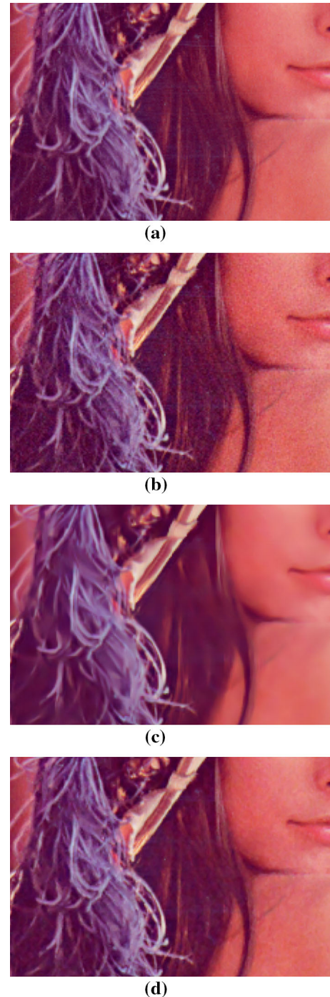
Fig. 25 a Original sub-image, b noisy sub-image, c denoised sub-image by FNLM, and d denoised sub-image by ANRAD
