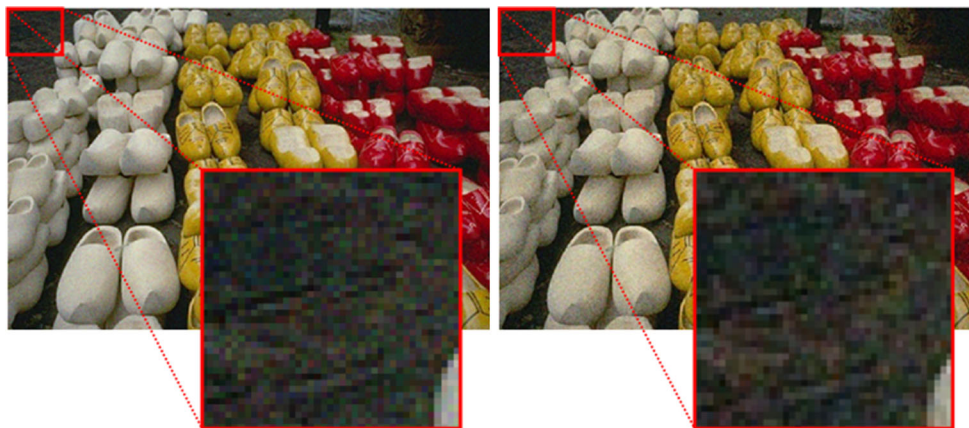
Fig. 2 Effect of demosaicing. Noisy image: left without demosaicing, right with demosaicing
