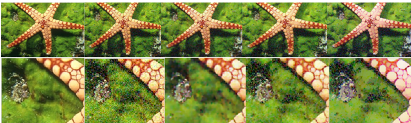
Fig. 19 Result of our filter on loaded image from Berkeley database (12003.jpg). The first row original image; image corrupted with color noise ( f(30), \sigma_c = 0.06 , and \sigma_s = 0.16 ), result of: ANRAD (SNR = 48.3407, iter = 40); DPAD (SNR = 41.1171, iter = 400) and SRAD (SNR = 39.5224, iter = 600). Second row corresponding zoomed images
