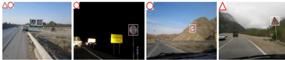
Fig. 5 Some results for shape classification of signs with different lighting conditions
