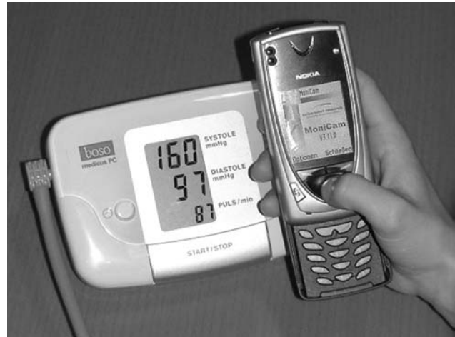
Fig. 2. a) "DiabDiary" – Java-based software application running on mobile phones supports the user in home-based data acquisition. b) "MoniCam" – principle: A special developed software helps the user in taking a photo of the display and sending it to a central monitoring centre via MMS, where the values are extracted and stored into the database
