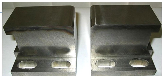
The left and right U-bend tool: 50 000 strokes without class 2 (< 2) U-bent sheet metal surface is the approval measure.
