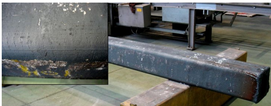
Fig. 9: First electrode cast with the modified graphite ring. Detail of the ingot angle surface
