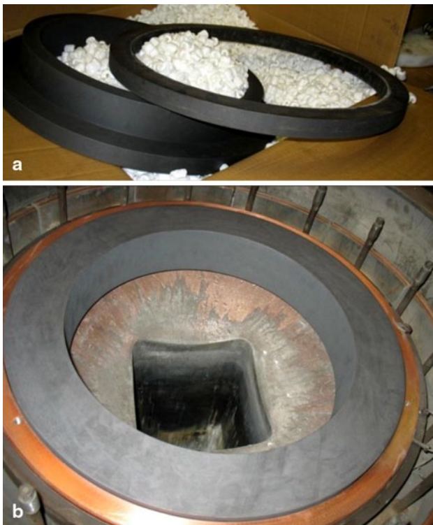
Fig. 6: a Modified and standard rings, b Experimental graphite ring put in place in the mould lower half
