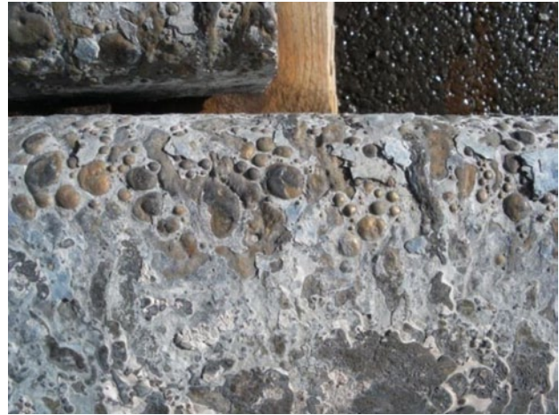
Fig. 1: Surface state obtained in one rare occasion, when the ingot was cast in "cold" metal meniscus conditions, on a specific grade with a low liquidus temperature
