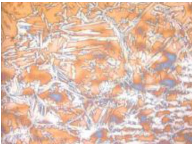
Fig. 10: Metallographic examination in HAZ of UR 2205 low ferrite
