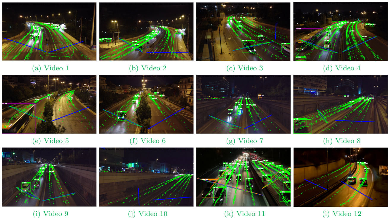
Fig. 4 Extracted vehicle trajectory data from the case study highways via the vehicle detection and the Bbox tracker
