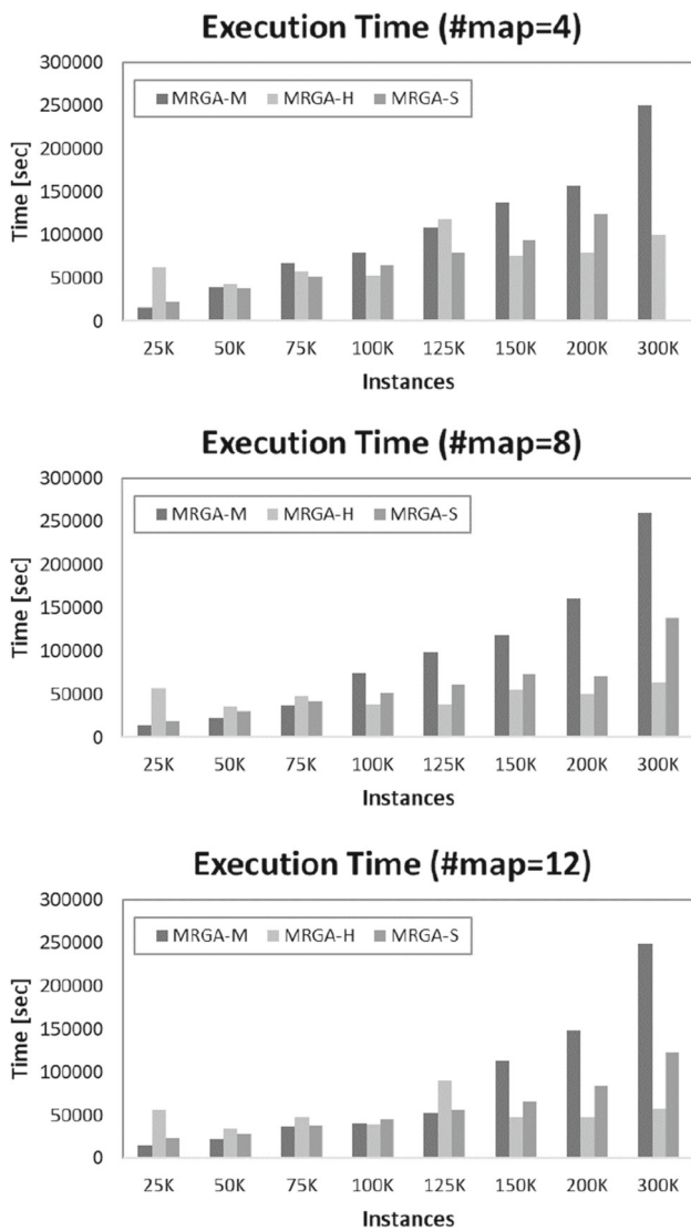
Fig. 7 Mean execution time of MRGA algorithms for each number of map tasks to solve the KP instances
