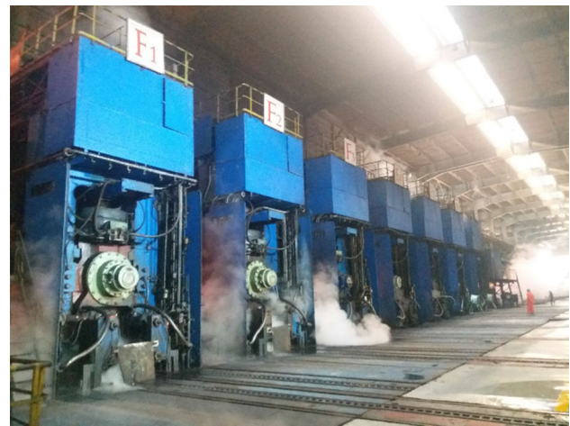
Fig. 4 Photograph of a real hot strip rolling mill at Chengsteel
