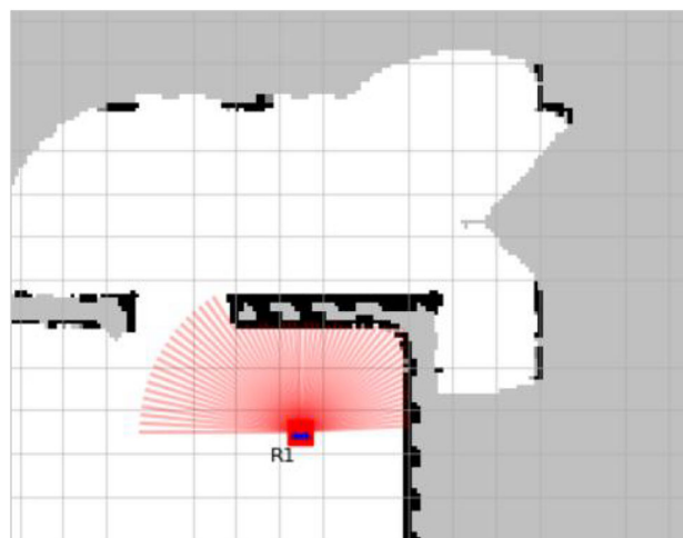
Fig. 1 An example of occupancy grid maps. White pixels represent the explored area; Gray pixels represent the unknown area; Black pixels represent the detected obstacles; Red lines represent the Laser sensor beams
