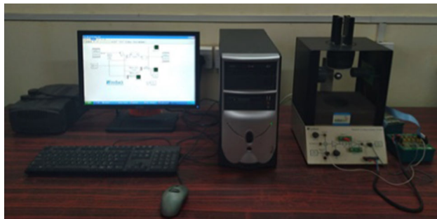
Fig. 36 Real-time control set-up of the Maglev system
